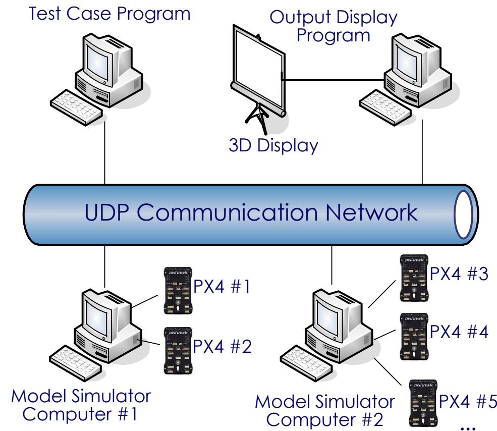
Fig. Structure of Multiple Flight Controllers Simulation
