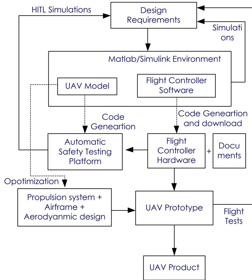
Fig. Structure of Mode-Based Design for UAV
