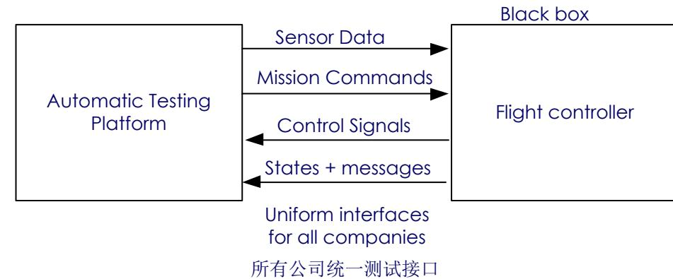
Fig. Structure of Multiple Flight Controllers Simulation
