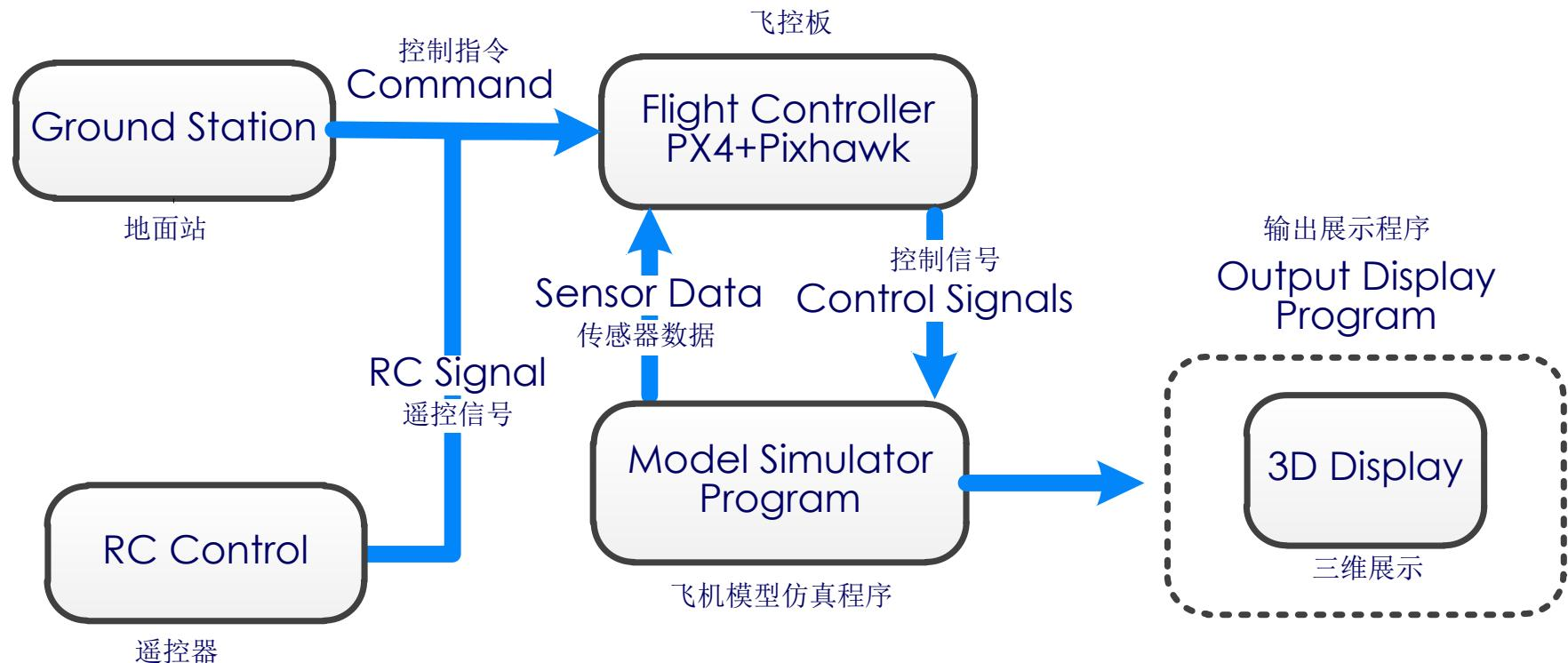
Fig. Flow Diagram of Normal Flight Simulation
