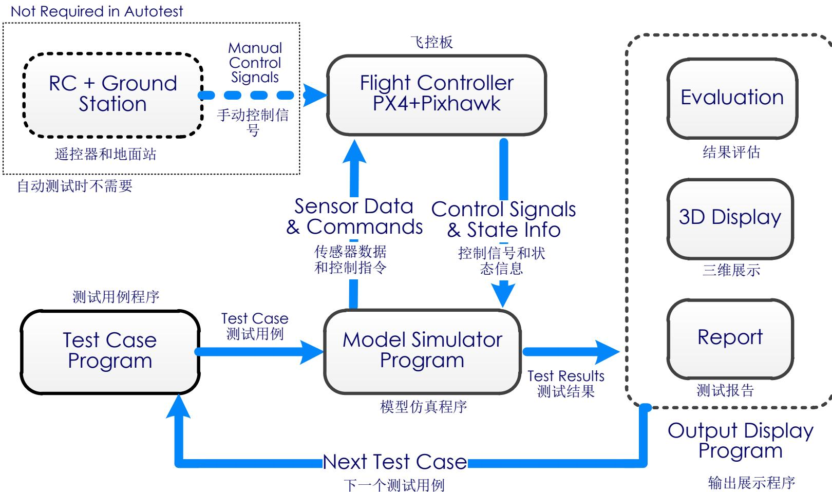
Fig. Flow Diagram of Safety Testing
