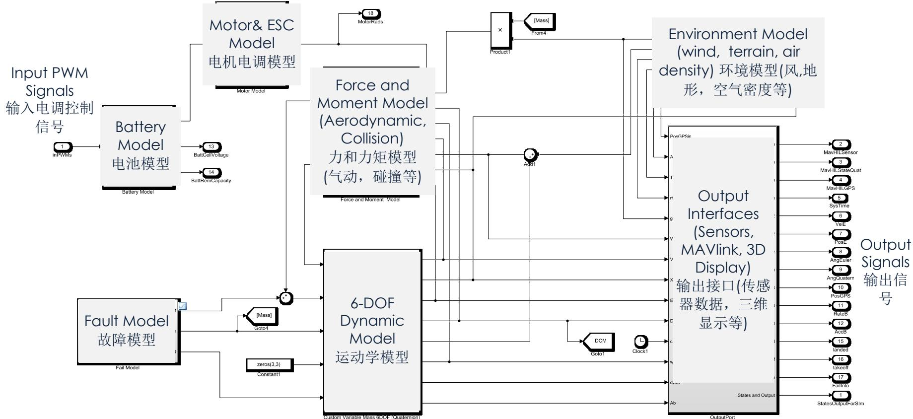
Fig. Structure of UAV Model Simulator in Simulink
