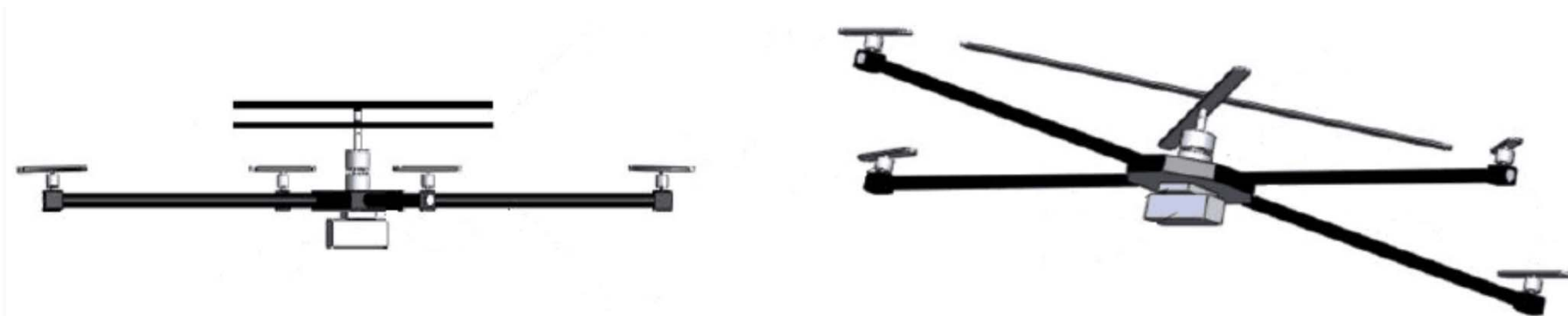
Figure 1.4 A compound multicopter. The middle coaxial rotor with a slow dynamic response provides the main lift, while the surrounding quadcopter can change the propellers' angular velocities rapidly to improve the dynamic response of attitude.
