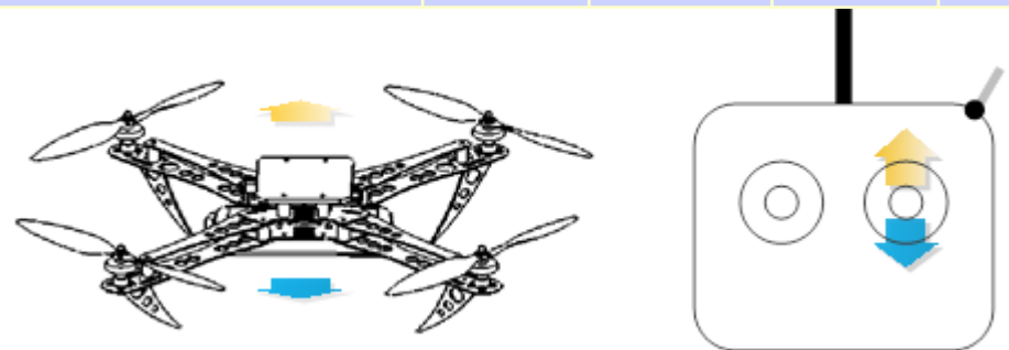
Figure 1.9 Operation of an RC transmitter for the forward and backward movement
