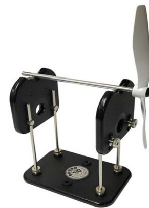
Figure 2.8 A Du-Bro propeller balancer
