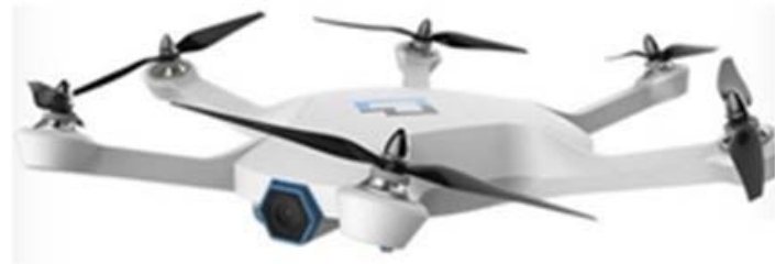
Fig 3.6 Non-horizontal disc Hexacopter CyPhyLVL1
