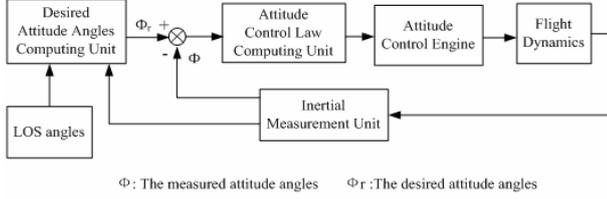
Fig. 4 Block diagram of KI attitude control system
