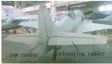
Fig. 1. Aircraft tail with elevating rudder and yaw rudder.
