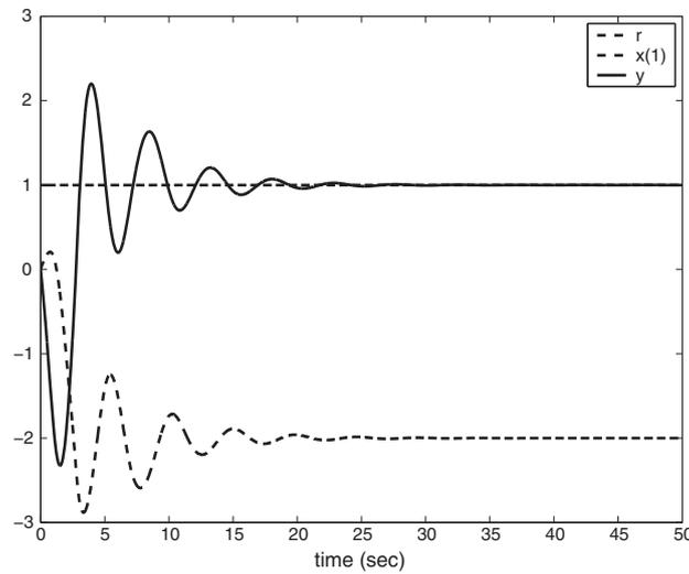
Figure 4. Time response of the nonlinear nonminimum phase system subject to a step disturbance.
