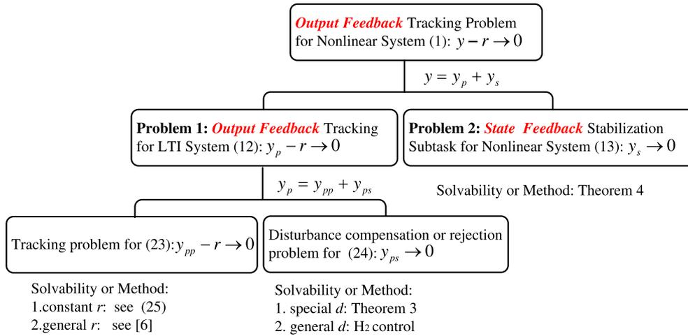
Figure 2. Additive state decomposition flow.
