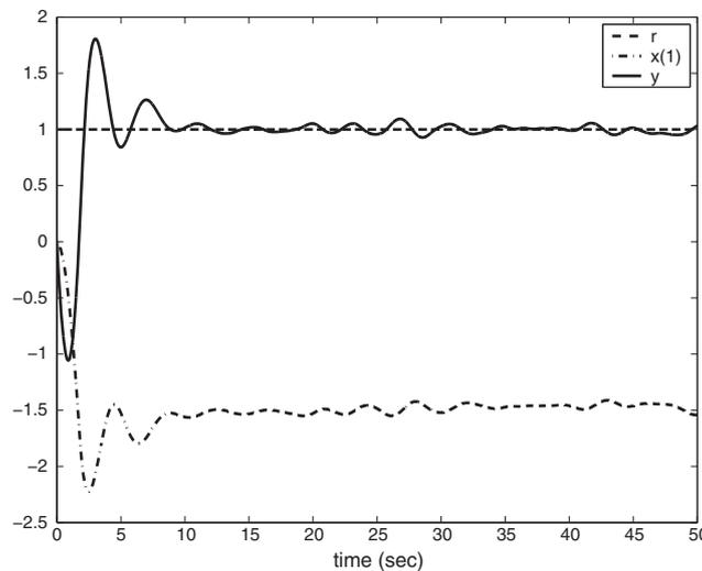
Figure 5. Time response of the nonlinear nonminimum phase system subject to a general bounded disturbance.
