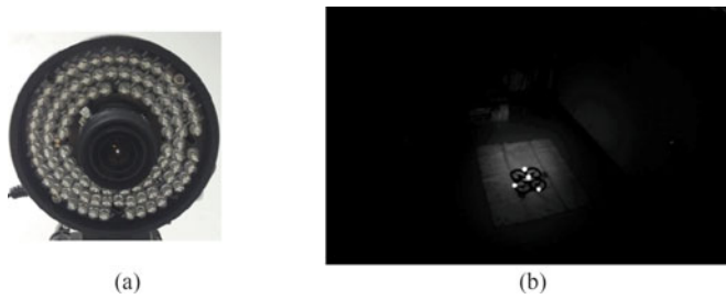
Fig. 8. (a) Infrared conventional camera and active LEDs; (b) sample image of the infrared conventional camera (exposure time is 34 ms).
