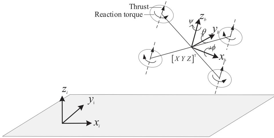
Figure 2. A dynamic scheme of the quadrotor.
