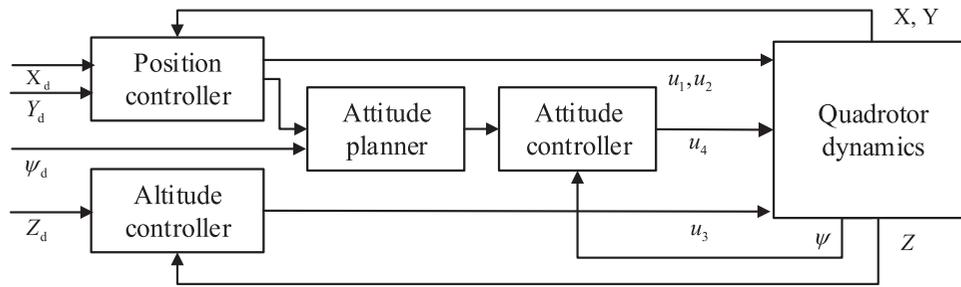
Figure 1. A hierarchical control scheme for autonomous trajectory tracking.
