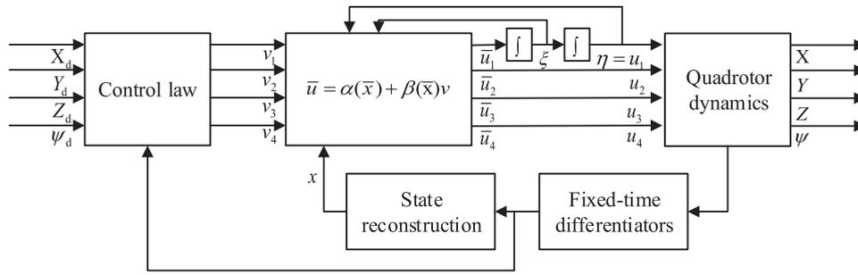
Figure 3. Observer-controller closed-loop system.
