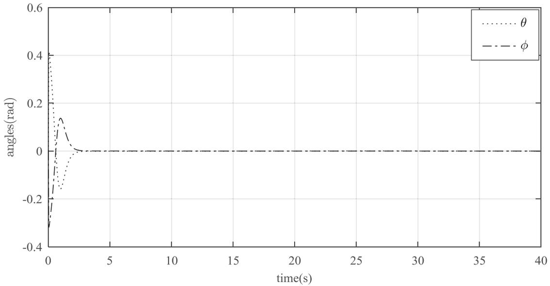
Figure 7. Pitch and roll angles.
