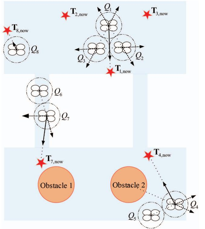
Fig. 3. A force diagram of multicopters in different states.
