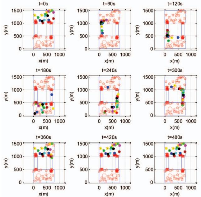
Fig. 6. The position of each multicopter in the same mission by using the designed protocol.
