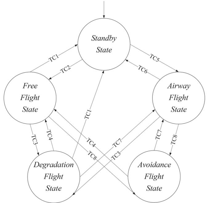
Fig. 4. Decision state machine for state selection of each multicopter.
