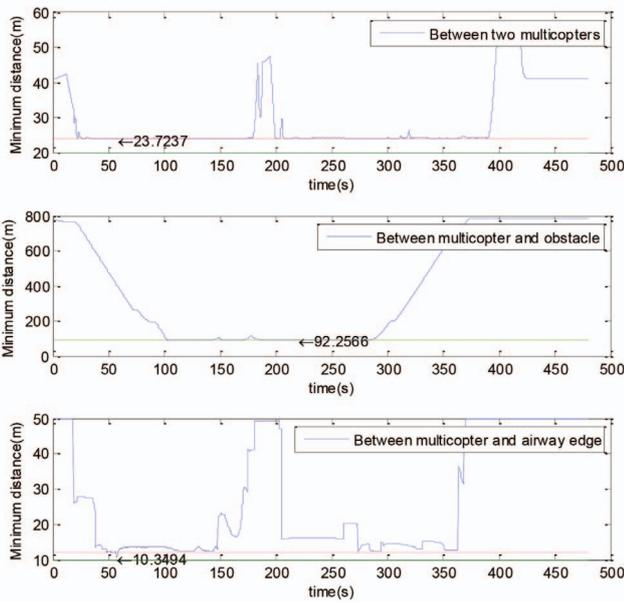
Fig. 7. Three kinds of minimum distance in the air traffic task by using the designed protocol.
