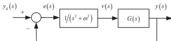
Figure: Sine signal tracking
