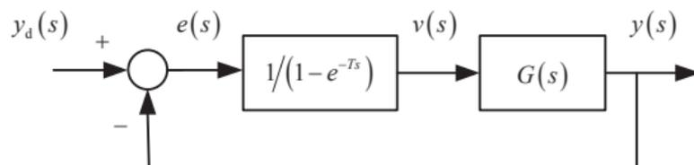
Figure: Periodic signal tracking of an RC system.
