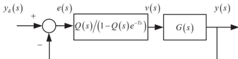
Figure: Periodic signal tracking of an FRC system.
