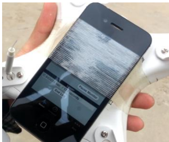
Fig.3 iPhone is fixed to the bottom of UAV
