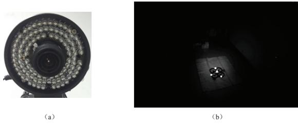
Fig. 8. (a) The infrared conventional camera and active LEDs; (b) A sample image of the infrared conventional camera (exposure time is 34 ms).
